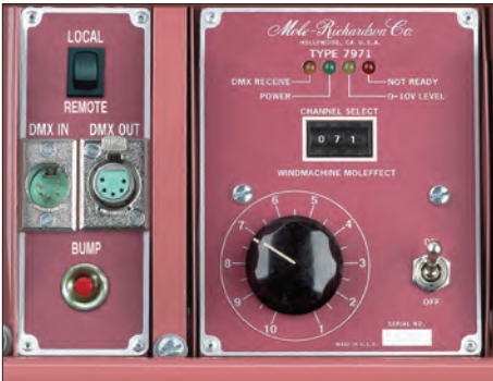
Close-up of DMX Control Panel
